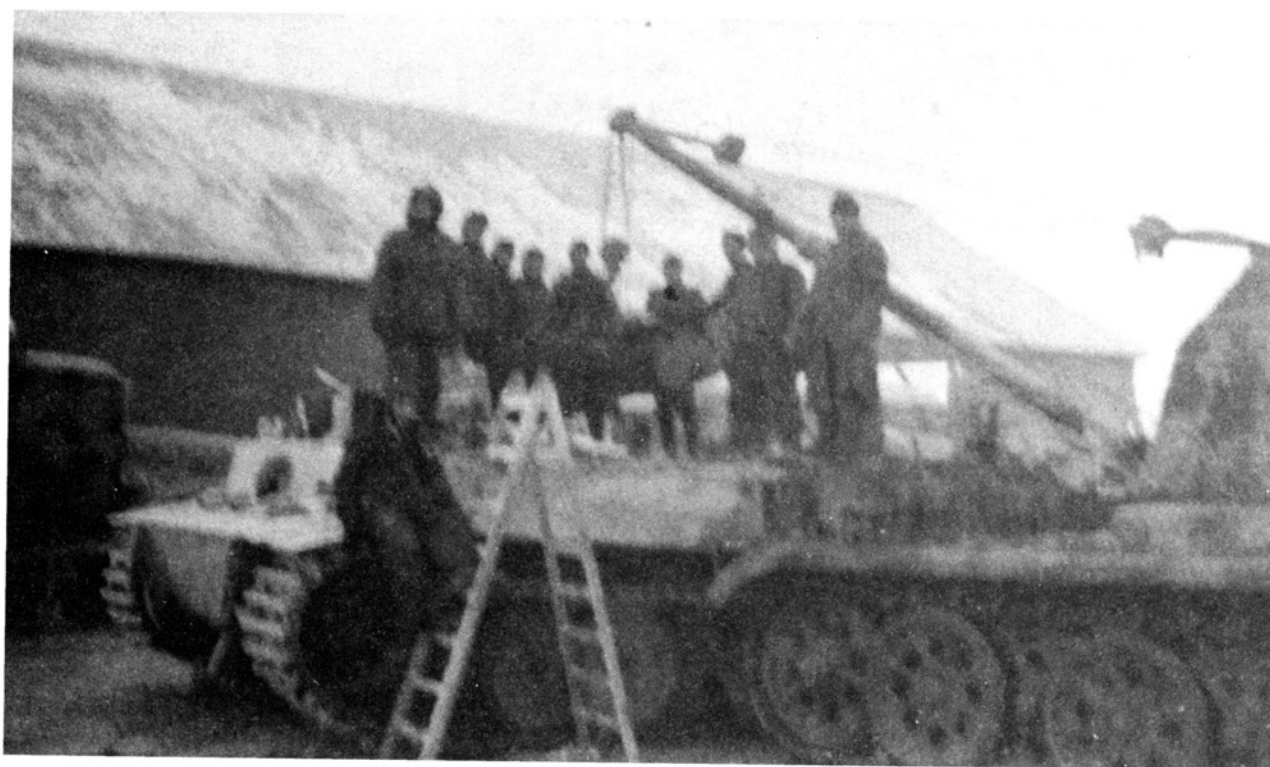
Maintenance is rarely mentioned in the after-action reports, but it is a major prerequisite for winning the battle. These photographs were taken at the end of the fighting around Bogoduchoff under cold-weather conditions. The 5-ton crane on the 18-ton prime mover can be seen to good advantage. It was used to remove engines and lesser loads from the Tigers; it was not suitable for lifting the turret. NÄGELE
