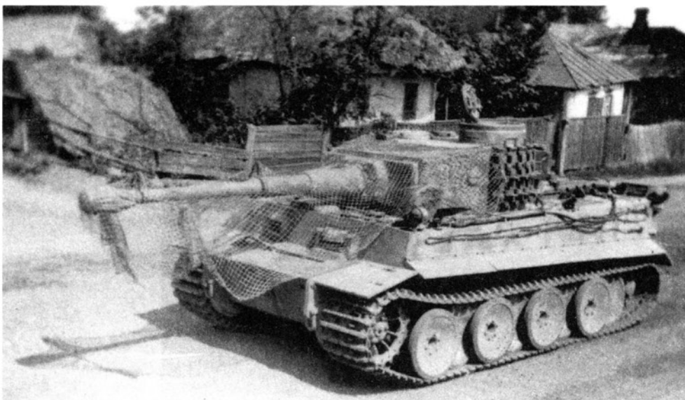
A small net has been used by the crew of the Tiger 932 to aid in camouflaging the tank by breaking up its outline. BENEKE
