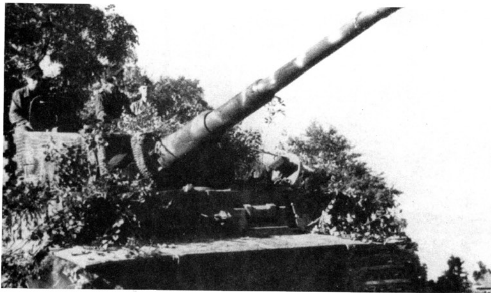
Tiger 211 in a camouflage scheme typical in Normandy: natural foliage. This was fine when stationary, but a moving "tree" is quite easy to spot from the air.
