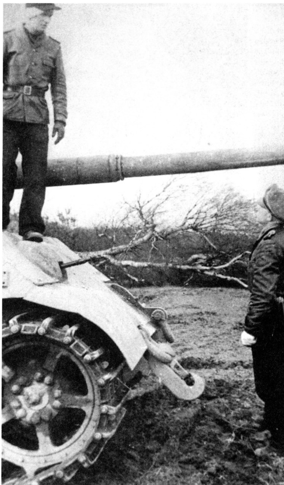
This photograph of the slightly wounded SS-Untersturmführer Bromann also clearly shows an interesting aspect of methods applied in the field. The double-ended hooks were left permanently attached to the tow shackles. This helped speed up the attachment of tow cables. The noncommissioned officer on the ground is SS-Oberscharführer Böde, the company's maintenance sergeant.
