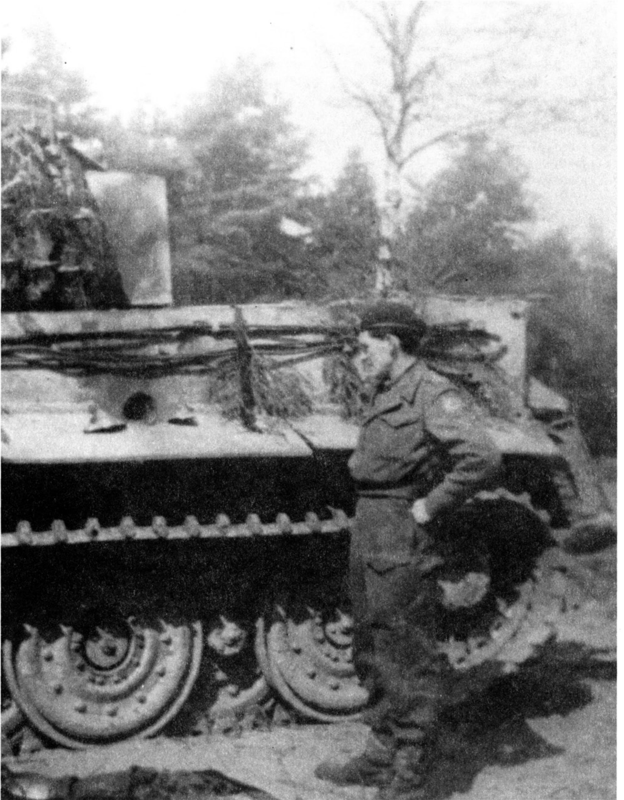
The Comet's hit is being examined by this British officer. Two fragments caused by the solid-shot projectile are visible on both sides of the penetration. The round hit the engine and brought the vehicle to a sudden stop.
