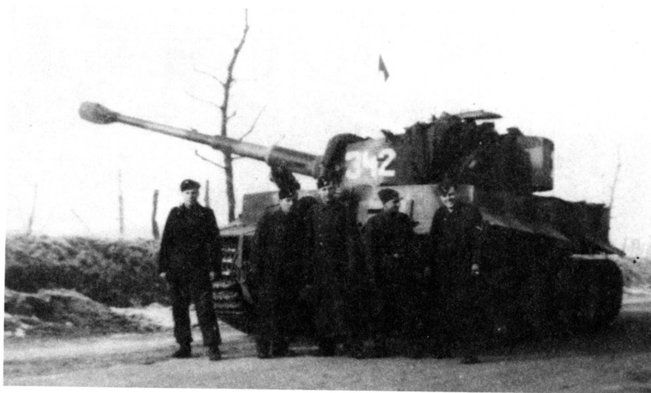
The 3./schwere SS-Panzer-Abteilung 101 had 18 tanks and used the overstrength vehicles to form a fourth platoon. In this photograph, we see Tiger 342 after it has broken down with a mechanical problem. The yellow flag on the top of the radio antenna makes it easier for the maintenance personnel to find the vehicle. WENDT
