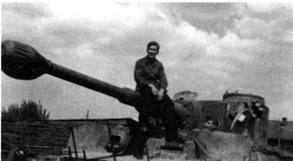
One of the older tanks, which still has the smoke-grenade launchers, has just received a set of additional track links on the front of the hull. The track pins still have to be hammered in; the crewmember assigned that task does not appear to be in too much of a hurry.
